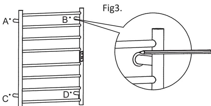
7. Mark the centres on the wall, note that the towel rail should be installed so that the bottom rail is at least 600mm above floor level.
