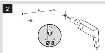
Use the drill with an appropriate drill bit to make holes at the marked places, and use a ceramic drill bit if the wall surface is made of ceramic tiles.
