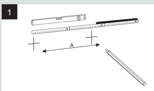
Using the hanging bracket and a spirit level mark the screw positions on the wall.
