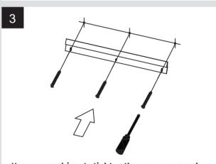
Use a screwdriver to tighten the screws securely affixing the hanging bracket to the wall.
