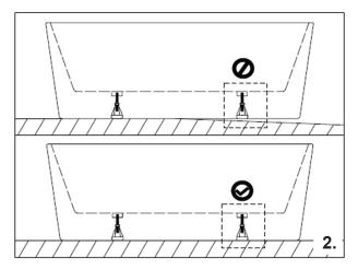
Check that bath sits flat; if required adjust legs to compensate for floor level. Once the bath has been levelled, ensure that the nut has been tightened on all feet.
