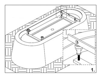
Assemble bath on a mat to protect against damage to bath surface. Ensure legs are adjusted in line with the base of bath. Ensure you have approximately 3-5mm of space between the bottom of the bath and finished floor surface. This prevents cracking of the bath shell. If the bath was to be installed hard against the floor the weight of water and the person/s having the bath can cause the bath to crack as there is no room for movement/flex.
