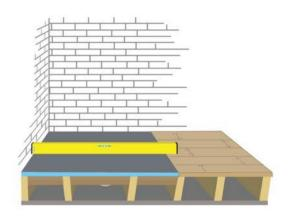
f. 19mm Floorboard/chipboard g. Floor joist (max 450 centres)
