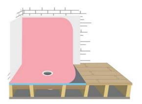
Apply an approved water proof membrane to the entire surface of the underlay, flange, water stop, and the wall sheeting according to the manufacturer recommendations.
