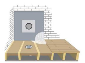
Make sure the shower tray system is fully supported. Use a polyurethane adhesive to fix directly to floor joist and noggins.
